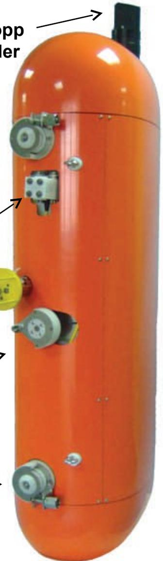
**Aqualog provides a researcher with homogeneous and regular time series of the vertical profiles of ocean quantities**
